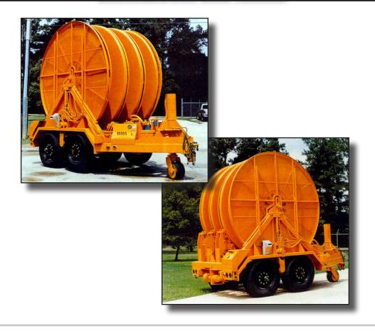
The TR-120-3 Underground Cable Reel Trailer is a 3 reel conductor payout trailer. With 9072 kg (20,000 lbs) of payload capacity, this trailer is ideal for users with a wide variety of underground conductor installation jobs. Load up with conductor and work in a number of locations. It's fast and convenient and its manoeuvrable.
